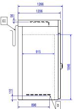
FΙ Electrical inlet (power) Refrigerant Outlet
